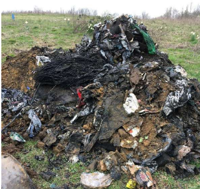
Photograph 41 – TP112 (shallow landfill material)
